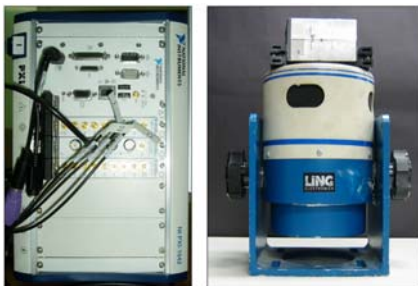
Fig. 2. PXI 4461 board generating excitation (left) and Exciter (right).
